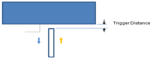
Picture: Proximity sensor triggering distances assessment Bottom Edge
