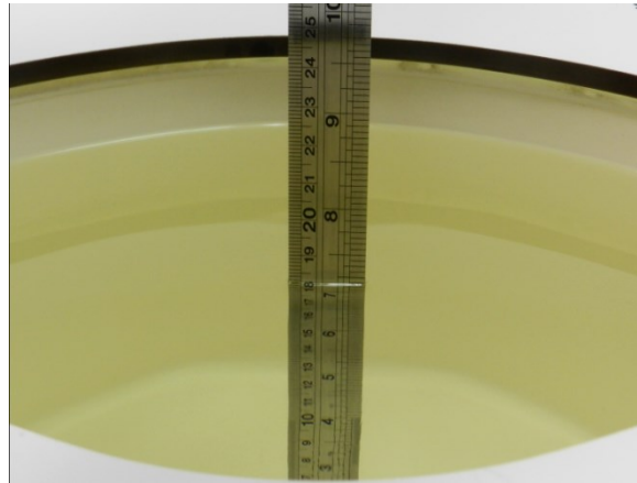
Fig 11.1 Photo of Liquid Height for Body SAR
