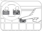
The camera button is connected to the water drainage hole on the back of your HONOR MagicBook Pro. If you accidentally spill water onto the camera, it will drain out from the drainage hole.
