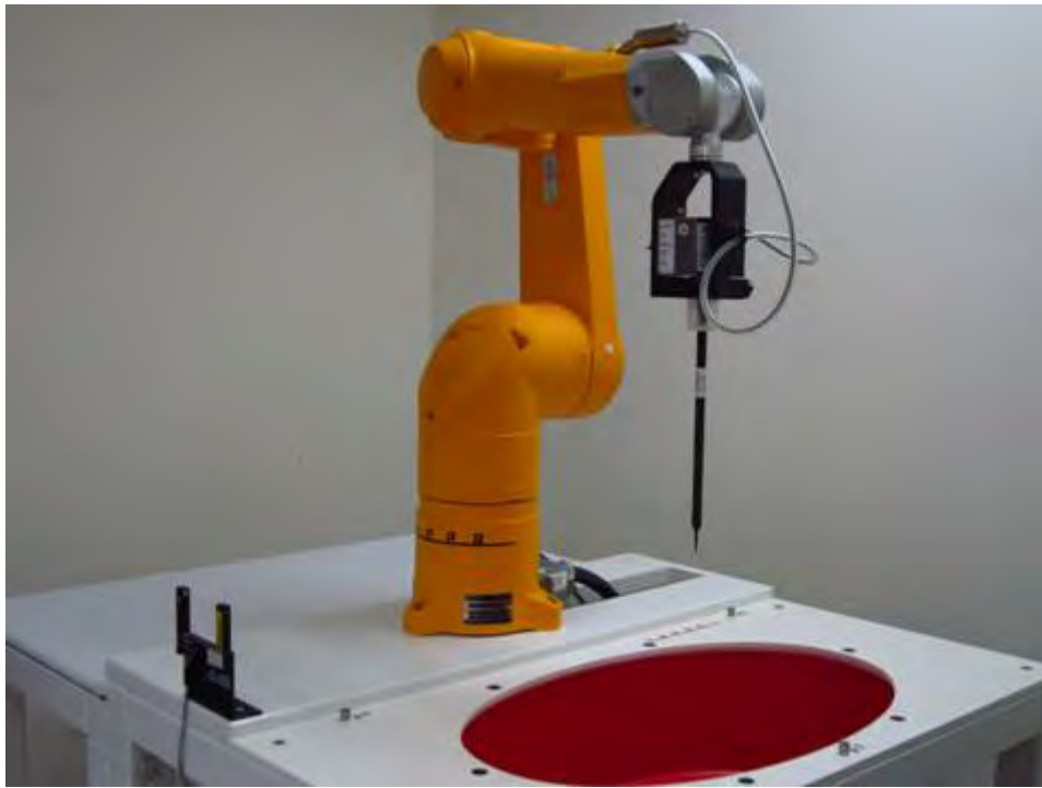
Fig.1 Photograph of the SAR measurement system
