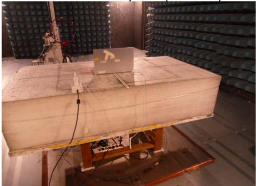
Radiated Emission Set up Photos (Below 1GHz)
