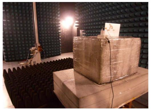
Radiated Emission Set up Photos (Front View)
