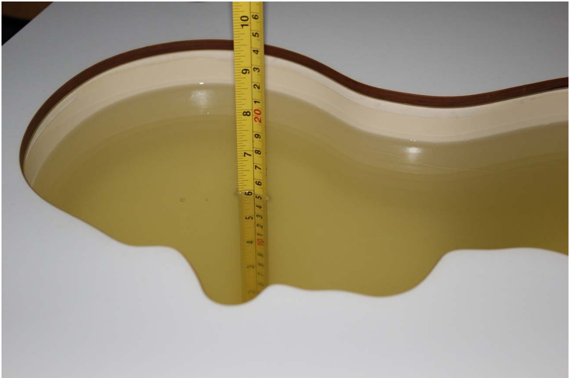
Picture 7-13 Liquid depth in the Head Phantom (2300 MHz)
