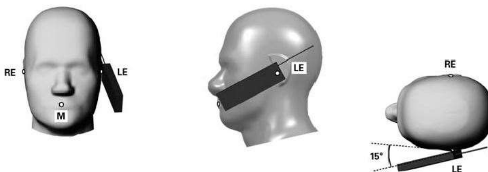
Fig 11.3.1 Tilt position. The reference points for the right ear (RE), left ear (LE), and mouth (M), which define the Reference Plane for handset positioning, are indicated.
