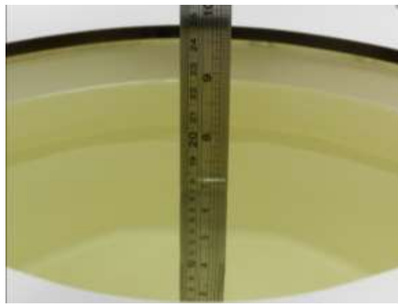
Fig 10.2 Photo of Liquid Height for Body SAR
