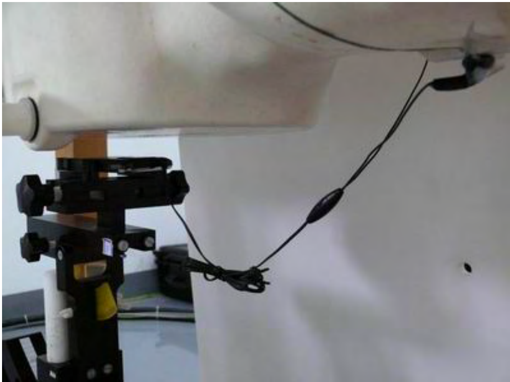
Picture 13: Body with earphone, The EUT display towards ground, the distance from handset to the bottom of the Phantom is 20mm)
