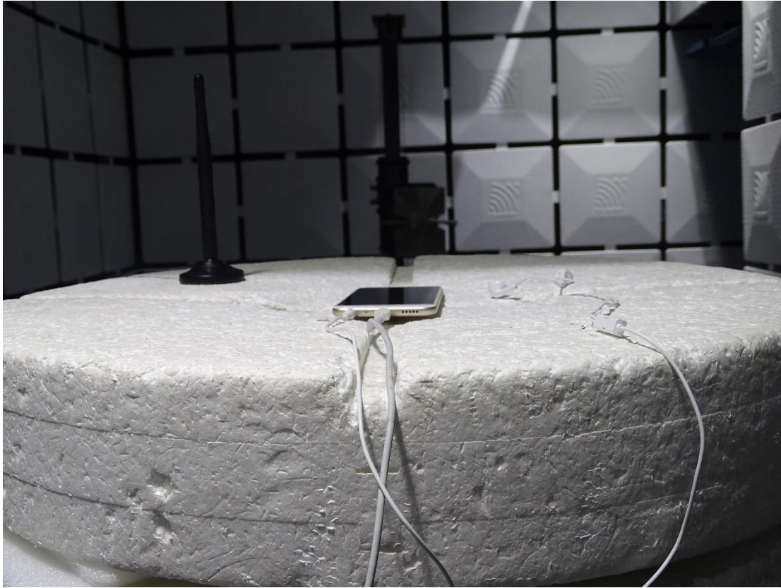
Radiated Spurious Emission (3GHz to18GHz)
