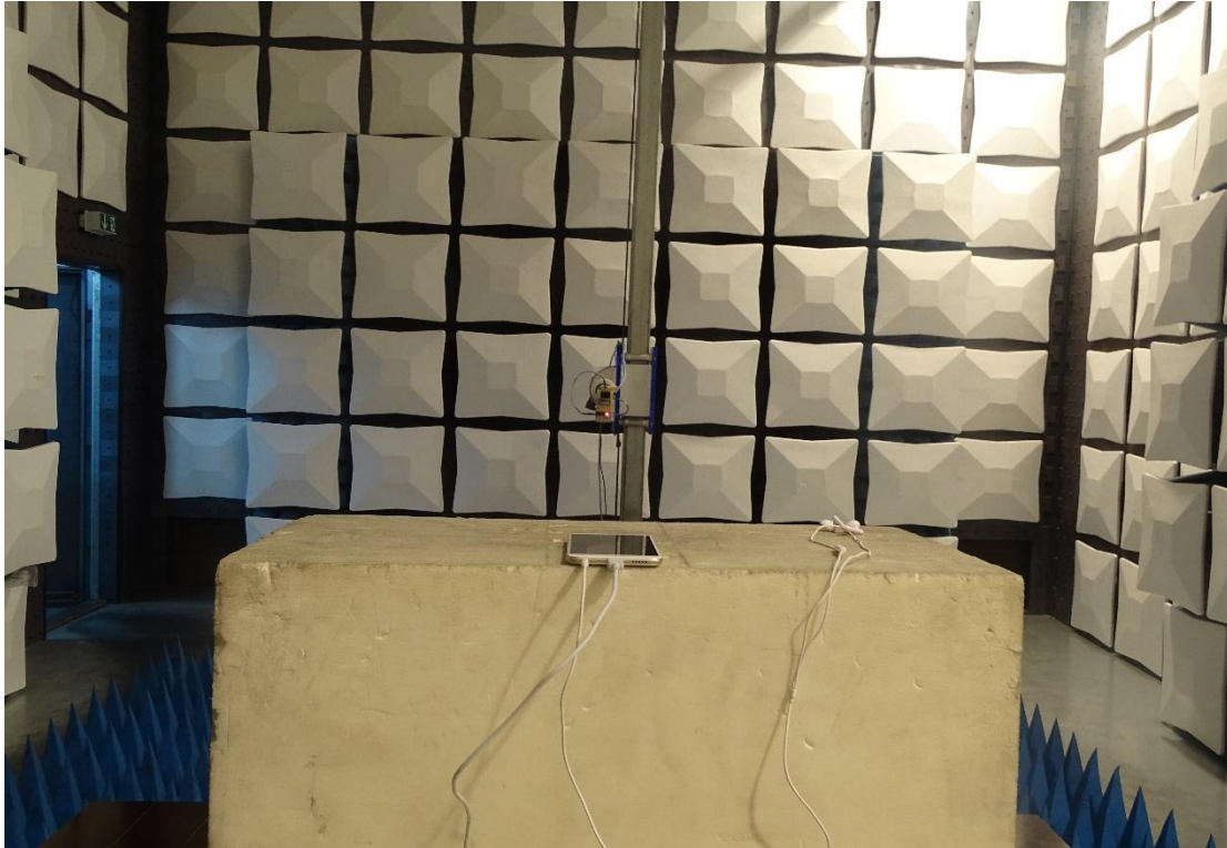
Radiated Spurious Emission (above 18GHz)
