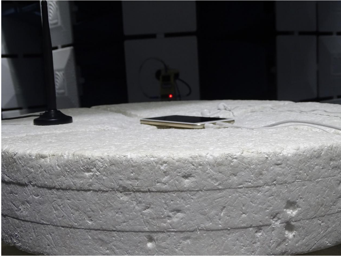
Radiated Spurious Emission (18GHz to26.5GHz)
