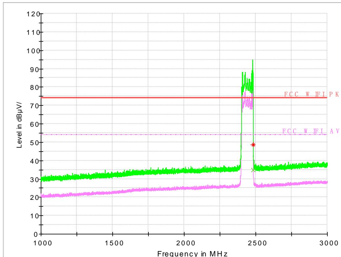
Note: The peak exceeds the limit line is carrier frequency.
