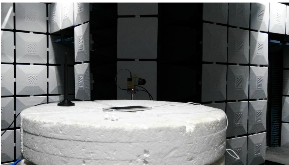
Radiated Spurious Emission (18GHz to26.5GHz)
