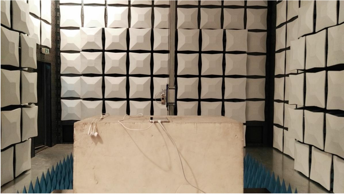
Radiated Spurious Emission (above 18GHz)
