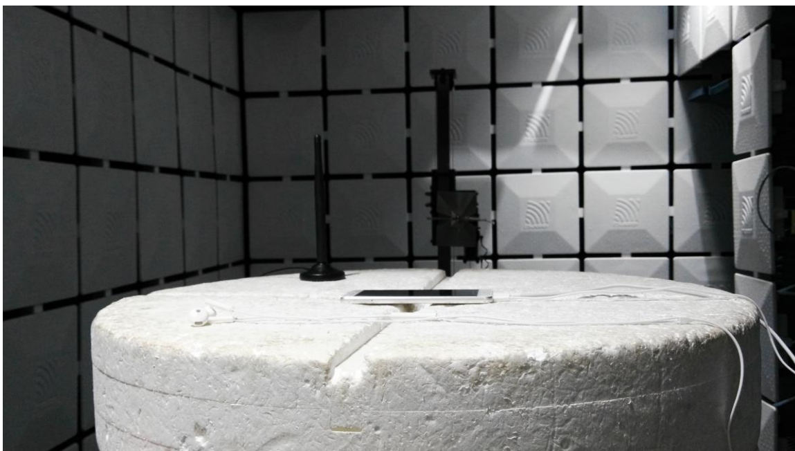
Radiated Spurious Emission (1GHz to18GHz)
