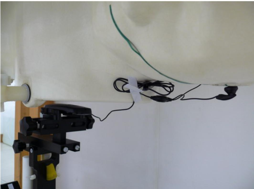
Picture 10 Body with earphone, towards the ground, the distance from handset to the bottom of the Phantom is 15mm)
