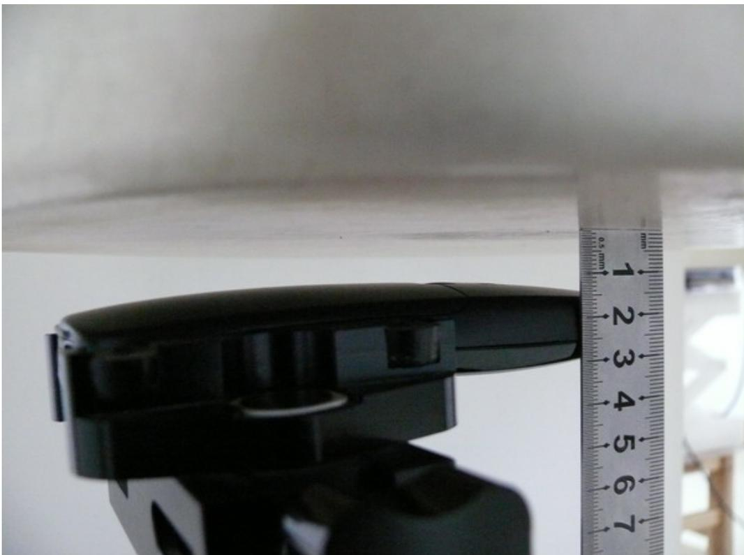
Picture 8: Body, The EUT display towards ground, the distance from handset to the bottom of the Phantom is 15mm)
