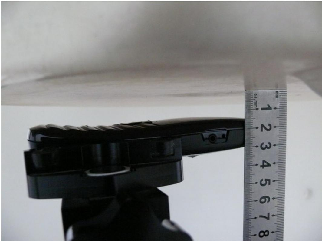
Picture 9: Body, The EUT display towards the Phantom, the distance from handset to the bottom of the Phantom is 15mm)
