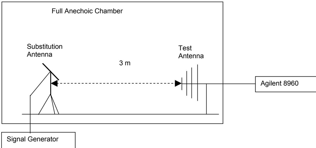
Figure 1. Test Set-up
