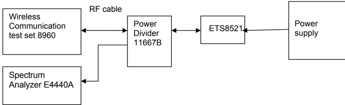
Figure 6. Test Set-up
