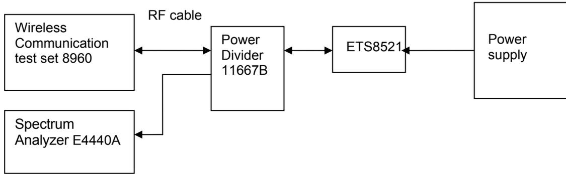
Figure 5. Test Set-up
