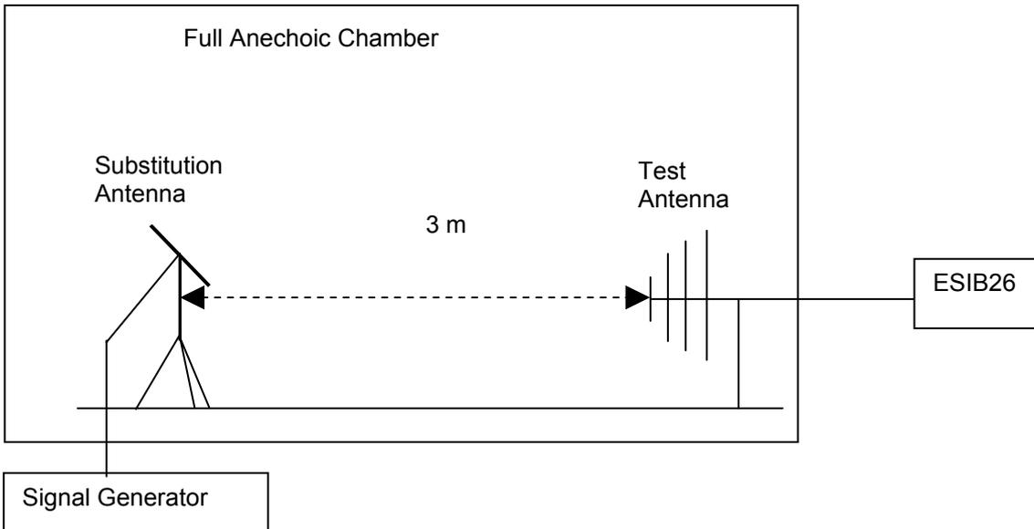
Figure 7. Test Set-up
