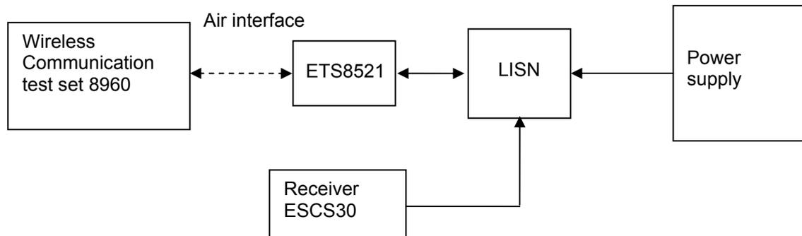
Figure 11. Test Set-up
