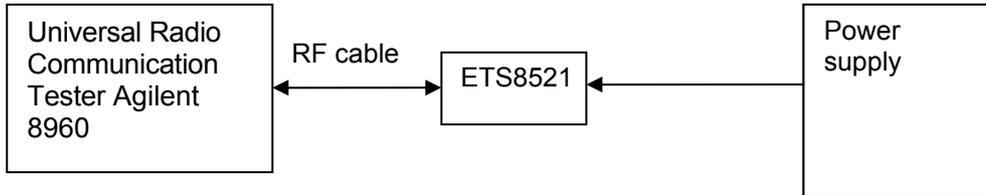
Figure 2. Test Set-up
