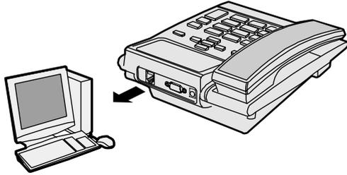
Connect the one end of the data cable to PC and the other end to the FWT. Fasten the captive screw to ensure reliable connection.
