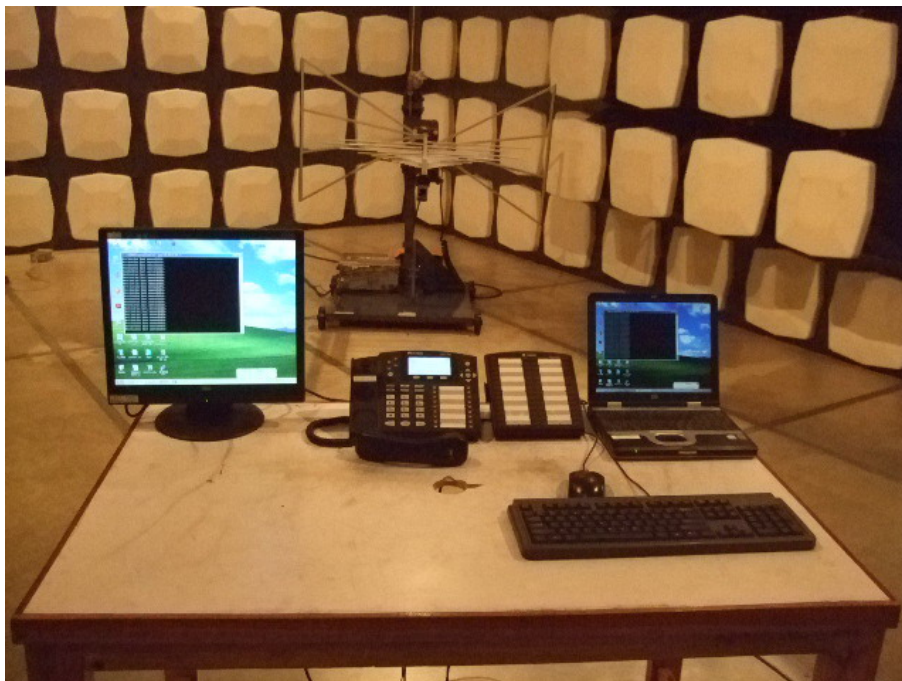
Radiated Emission Test Set-up(Below 1GHz)
