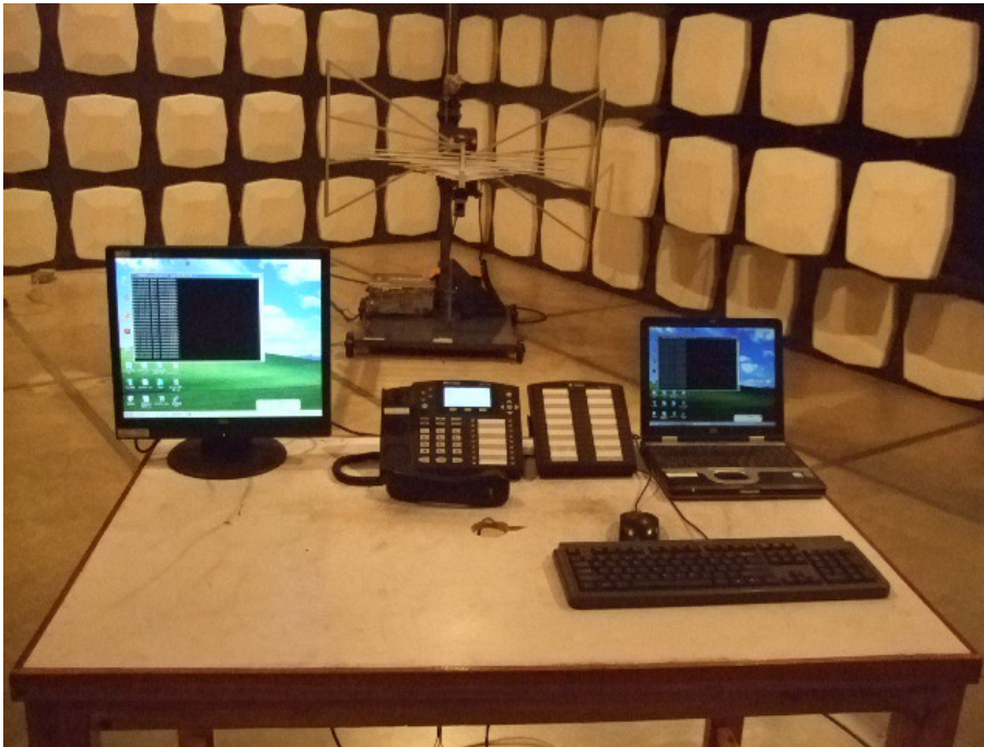
Radiated Emission Test Set-up(Below 1GHz)
