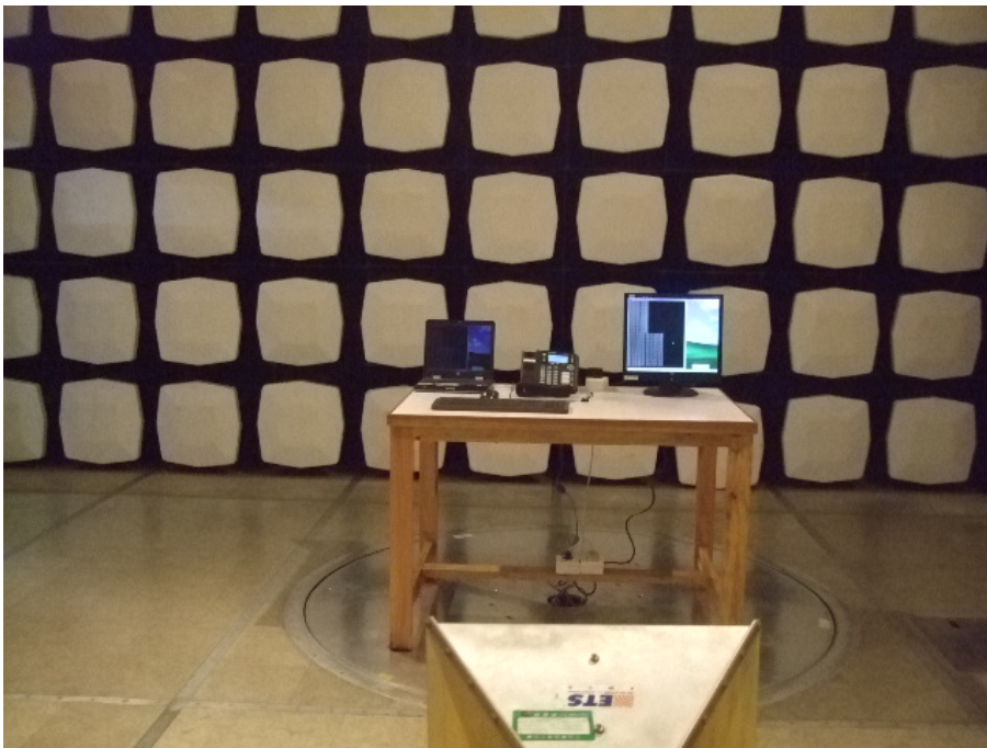
Radiated Emission Test Set-up(Above 1GHz)
