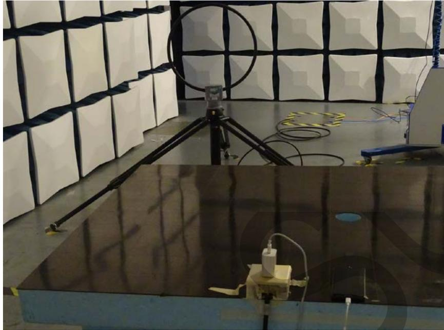
Radiated Disturbance Emissions (9Khz-30Mhz)
