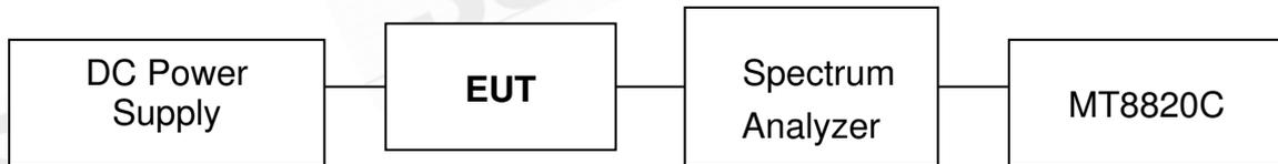
**Fig. 2-2 Configuration of Tested System (Fixed Channel-Radiated)**
