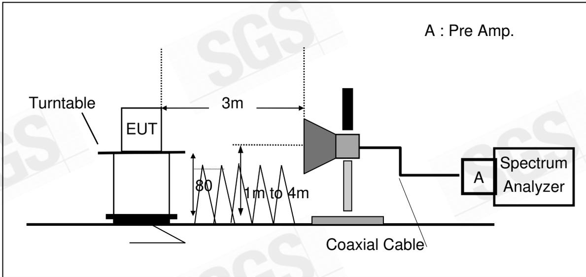
(C) Substituted Method Test Set-UP
