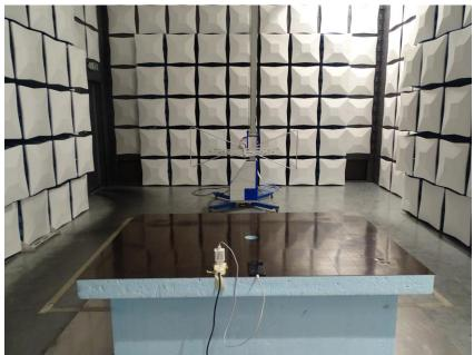
Radiated Disturbance Emissions (30Mhz-1GHz)
