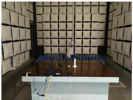
Radiated Disturbance Emissions (26.5GHz to 40GHz
