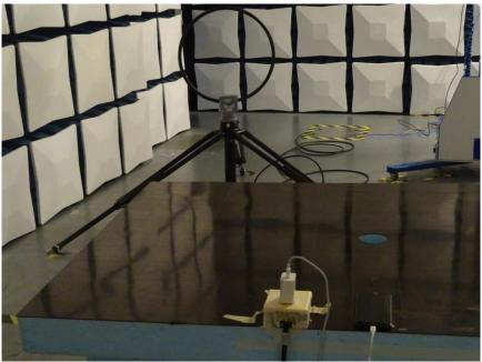
Radiated Disturbance Emissions (9Khz-30Mhz)
