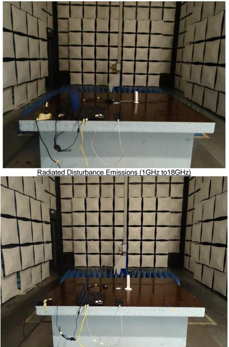
Radiated Disturbance Emissions (18GHz to 26.5GHz)
