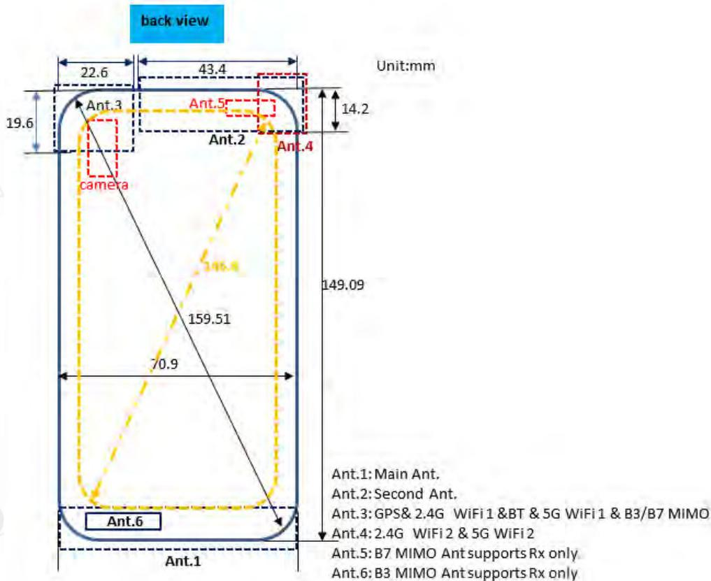
The test device is a mobile phone. The display diagonal dimension is 146.8mm and the overall diagonal dimension of this device is 159.51mm.
