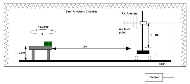
Figure 1. Test set-up of radiated disturbance(30MHz-1GHz)
