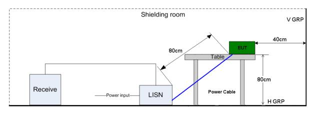
Figure 3. Test Set-up of conducted disturbance
