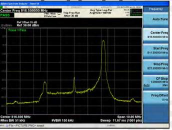
Part 90\_Band 26\_5M\_64QAM\_LOW\_RB25,0
