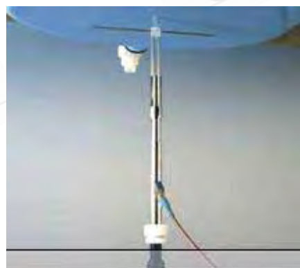
Photograph of the dipole Antenna
