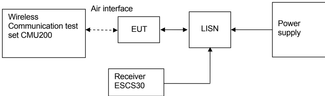
Figure 4. Test Set-up
