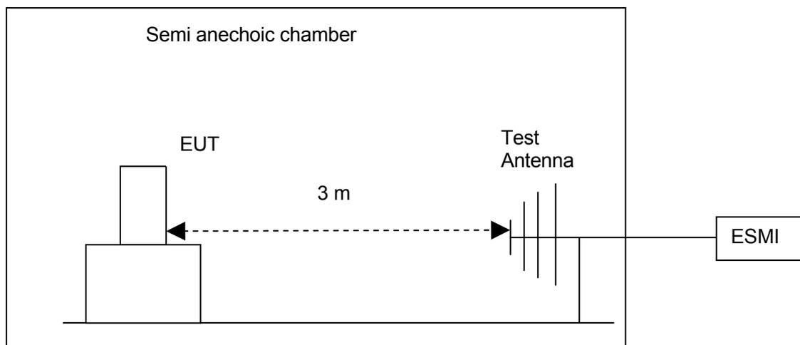
Figure 3. Test set-up
