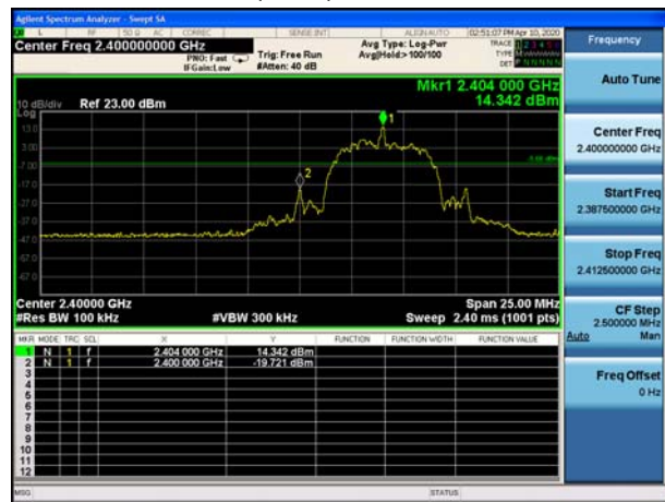
BT UHD 4M \pi/4 -DQPSK, Carrier frequency (MHz): 2404
