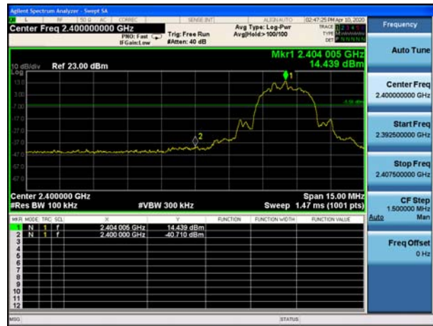
BT UHD 4M \pi/4 -DQPSK, Carrier frequency (MHz): 2404
