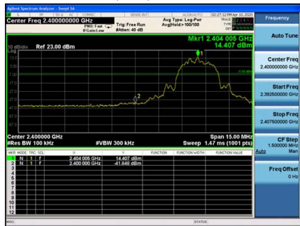
BT UHD 2M 8DPSK, Carrier frequency (MHz): 2404
