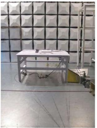
Radiated emission for 1GHz to 18GHz
