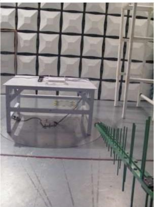
Radiated emission for 30 MHz-1 GHz
