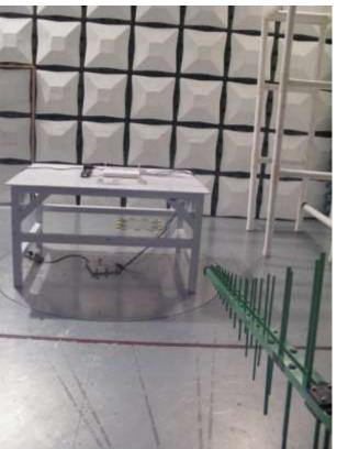
Radiated emission for 30 MHz-1 GHz
