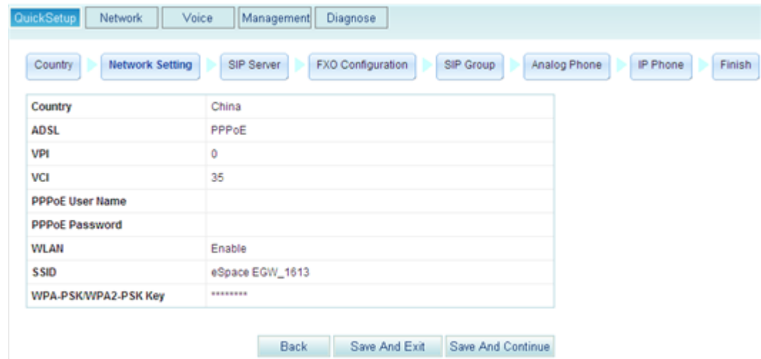
Figure 6-4 Network configuration complete
