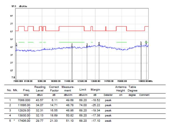
Note: 1. Measurement = Reading Level + Correct Factor.
