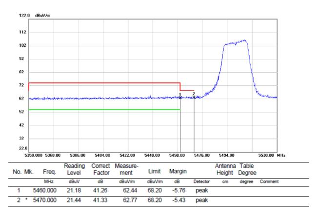
Note: 1. Measurement = Reading Level + Correct Factor.
