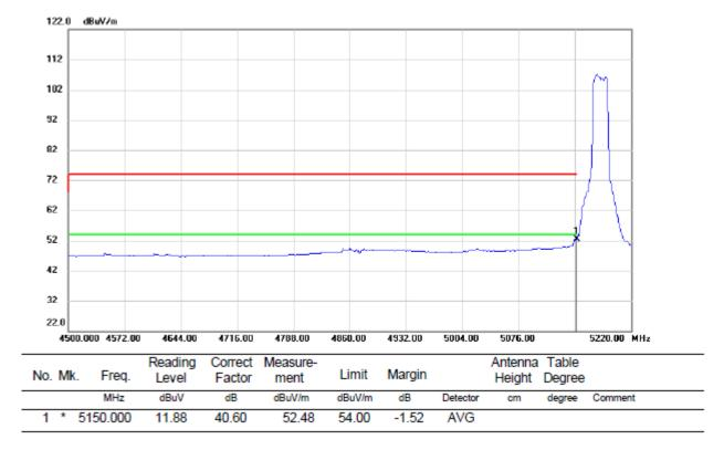
Note: 1. Measurement = Reading Level + Correct Factor.
