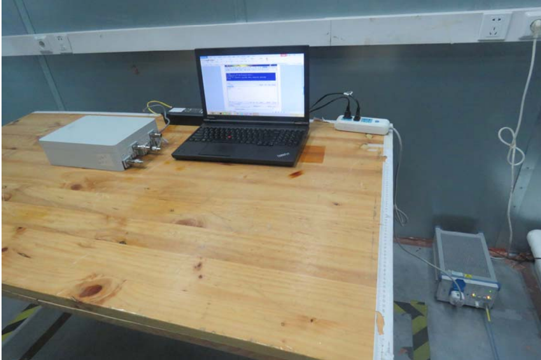
Picture 3 Conducted Emission Test Setup
