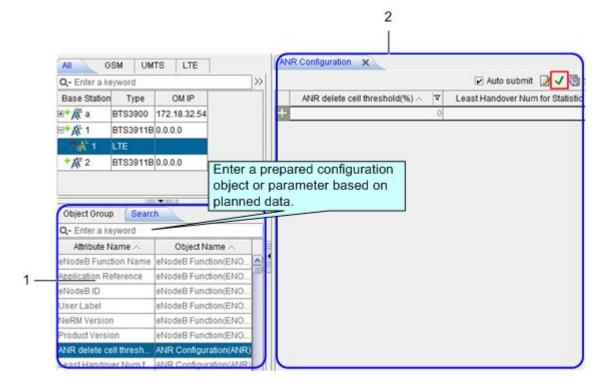
2. In area 1, select or search the MO to be configured based on the planned data and double-click the MO. On the displayed page as shown in area 2, set parameters as required, and click to save the parameter configuration.
