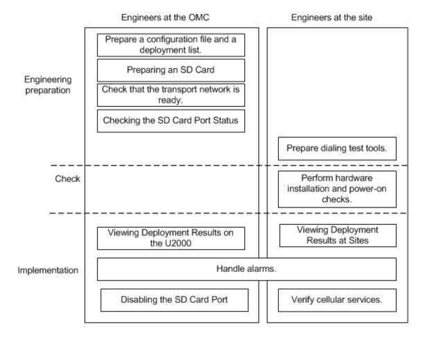
Figure 1-2 Site deployment process
