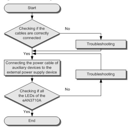
Figure 1-22 Power-on check procedure
