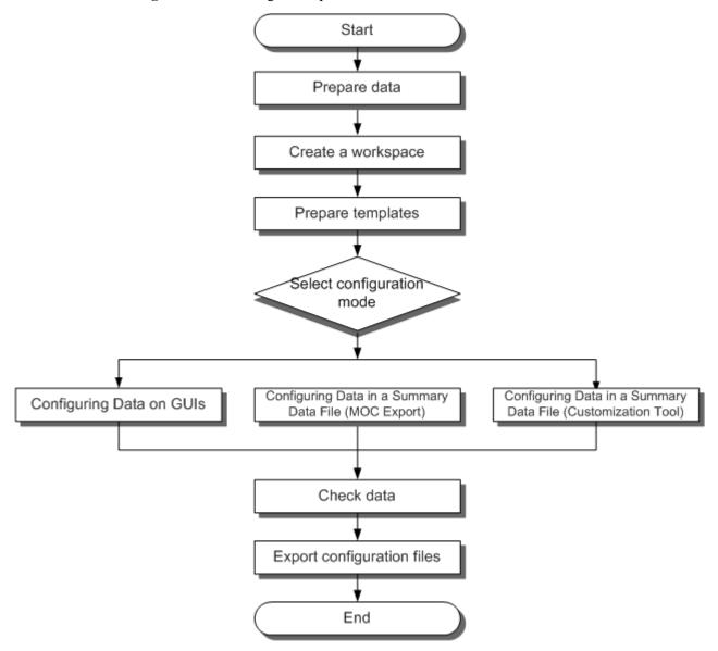
Figure 1-3 Data configuration process
