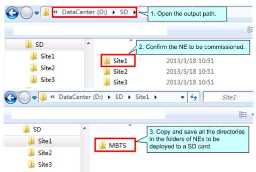
Figure 1-7 File copy procedure in One USB for One Site mode
