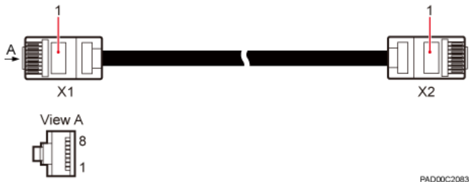
Figure 1-12 Ethernet cable exterior
