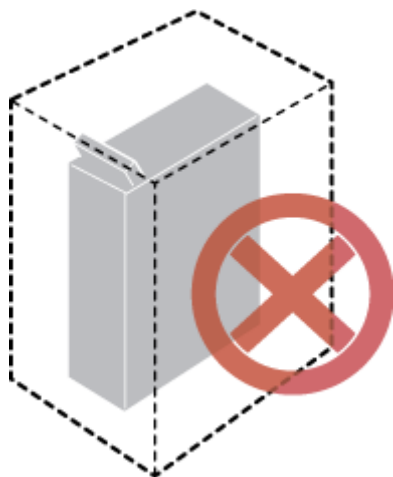
Figure 2-7 Inappropriately installed eAN3710A
