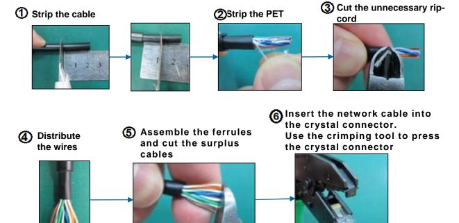
Notice: Donot press the outer-jacket into the crystal connector.
