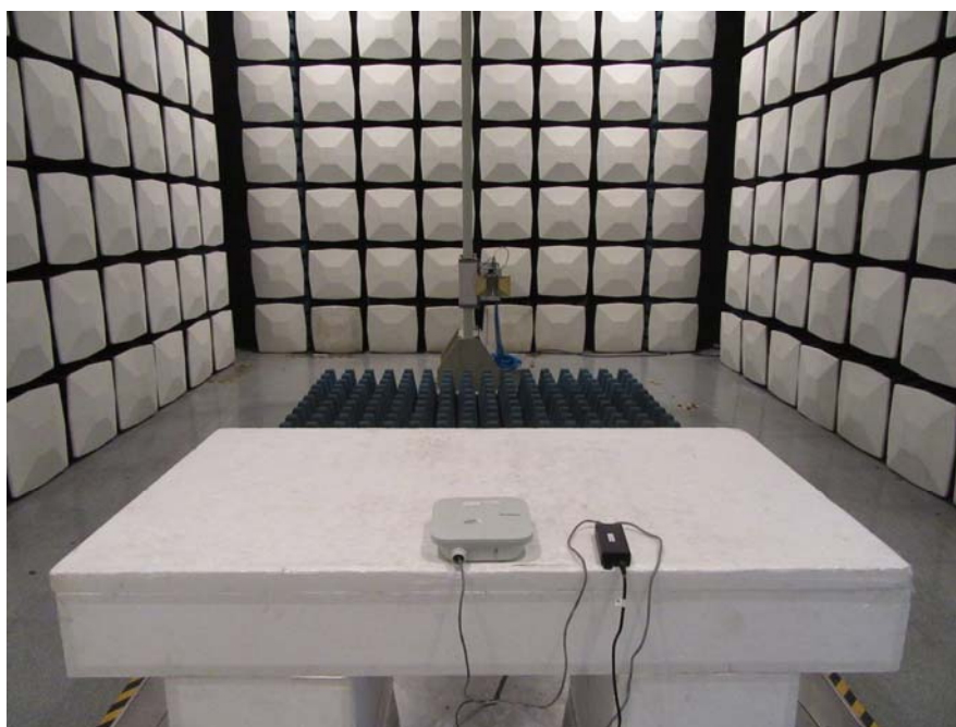
Radiated Emission Above 1 GHz - Rear View
