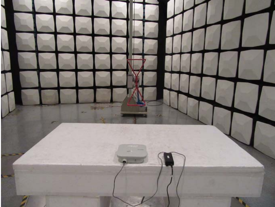
Radiated Emissions Below 1GHz - Rear View
