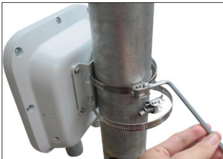
Figure 3-5 Adjusting the length of the hose clamp
