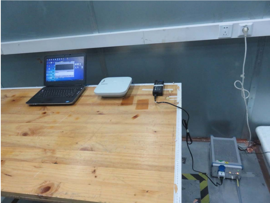
Picture 3 Conducted Emission Test Setup
