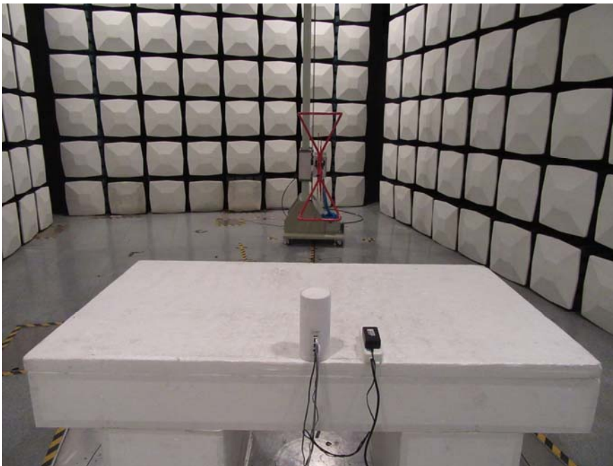
Radiated Emissions Below 1GHz - Rear View
