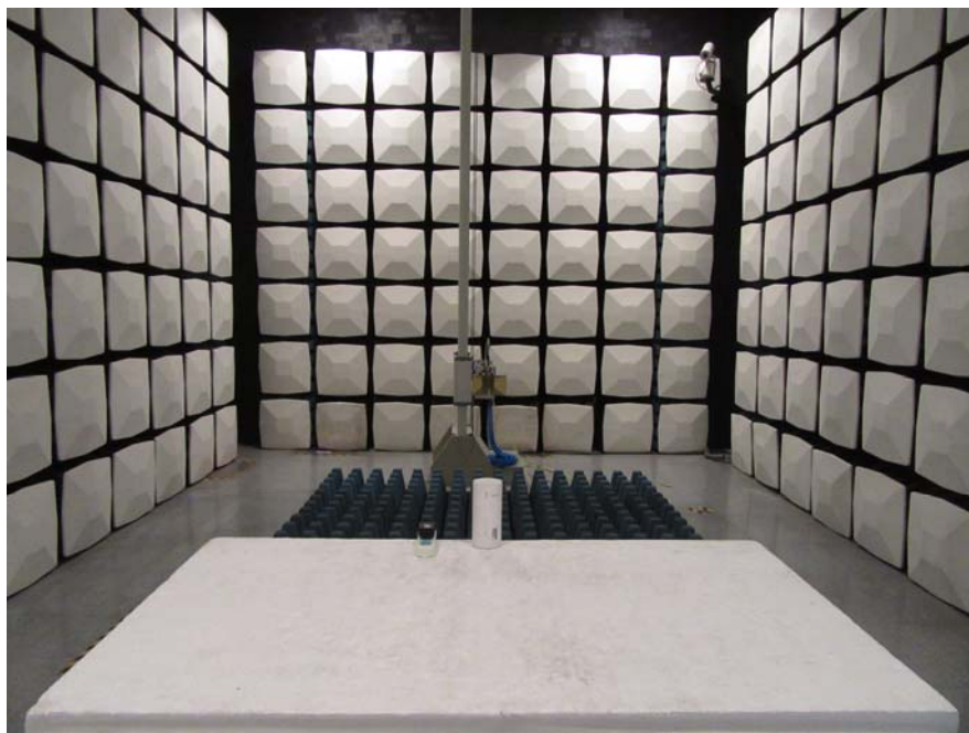
Radiated Emission Above 1 GHz - Front View
