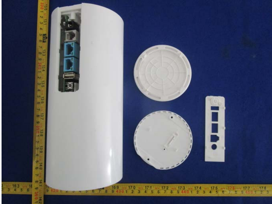
EUT – Cover Removed View
