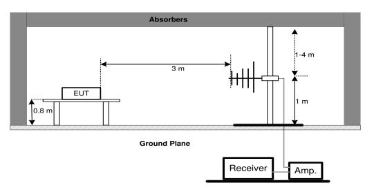
(B) Radiated Emission Test Set-Up Frequency 1 GHz
