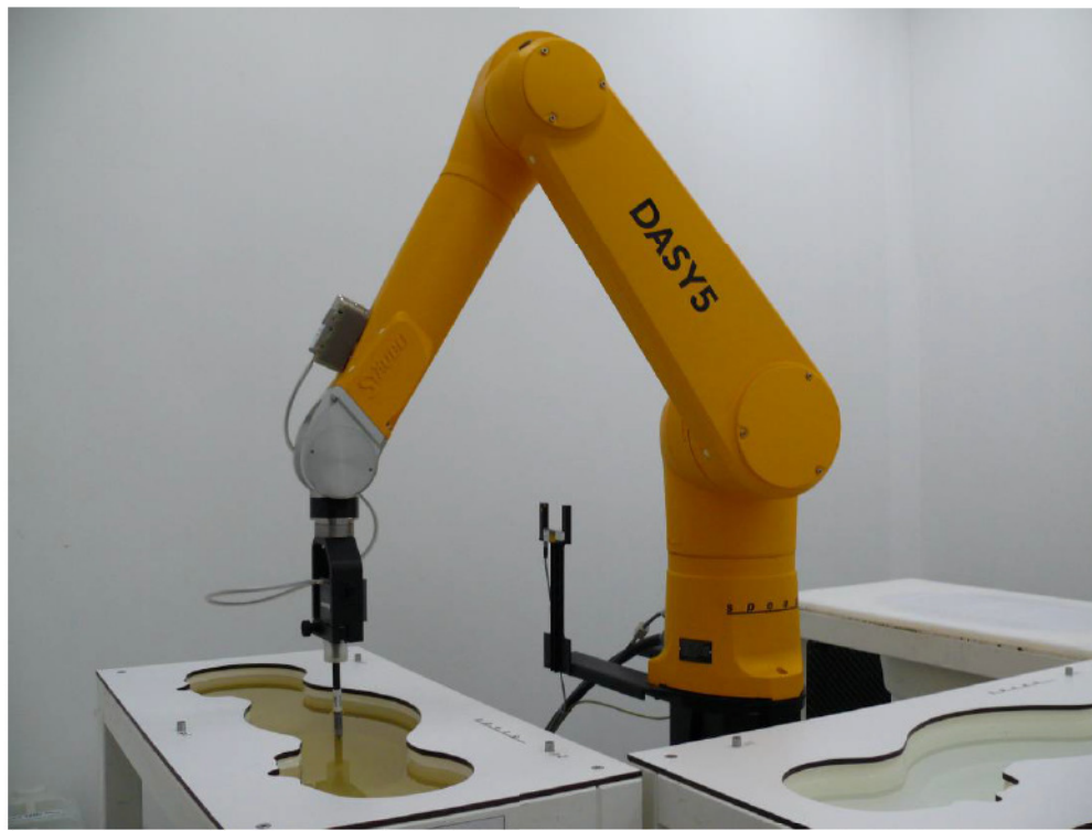
Picture 2: Specific Absorption Rate Test Layout
