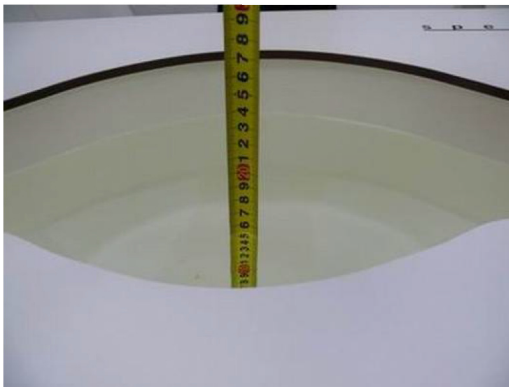
Picture 5: Liquid depth in the Flat Phantom (1900 MHz, 15.2cm depth)
