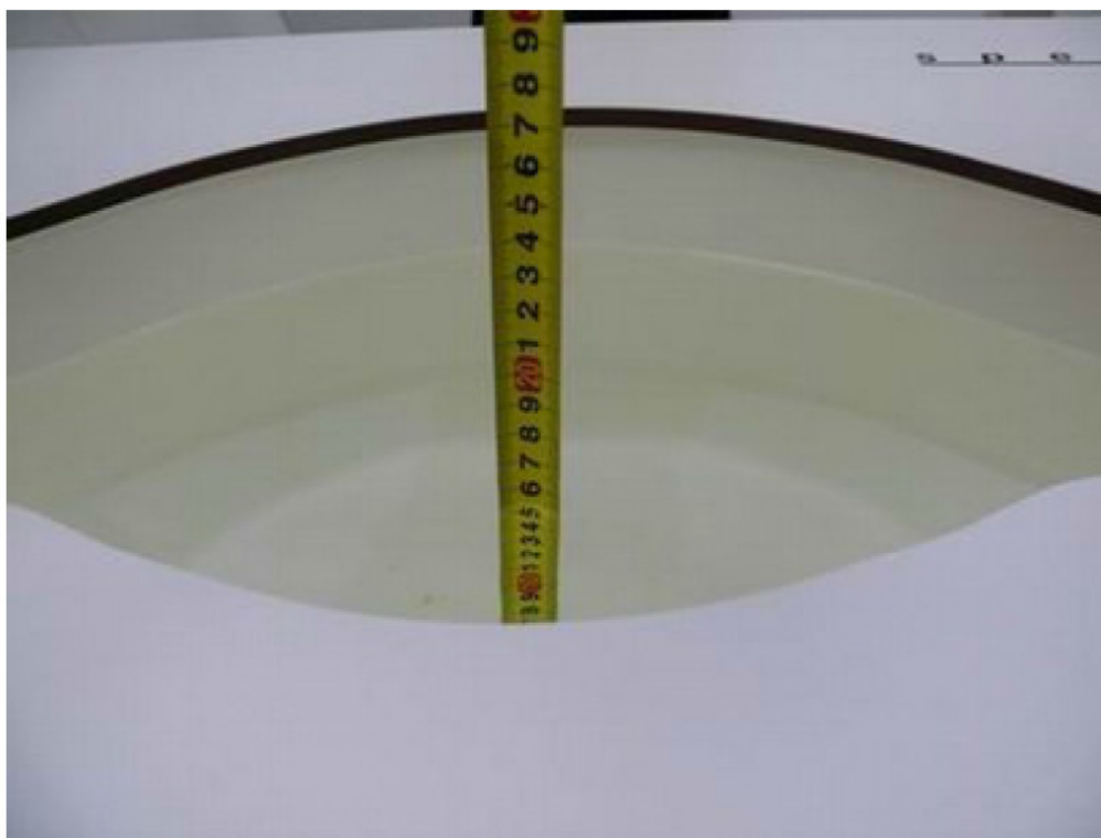
Picture 6: Liquid depth in the flat Phantom (2450 MHz, 15.3cm depth)
