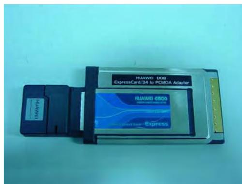
Picture 1-d: EUT inserted into ExpressCard/34 to PCMCIA Adapter
