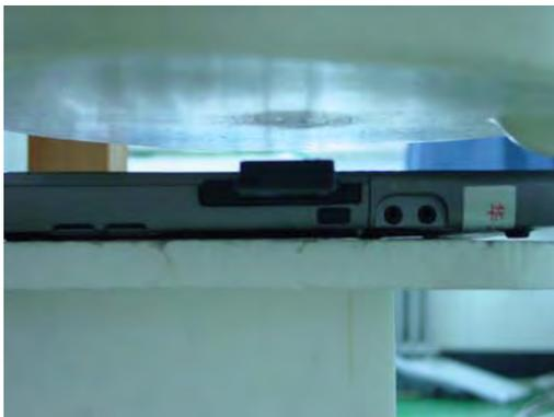
Picture 2-b1: Test position 2 with antenna folded
