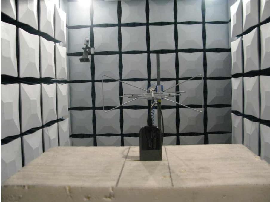
Radiated Spurious Emission (below 3GHz)
