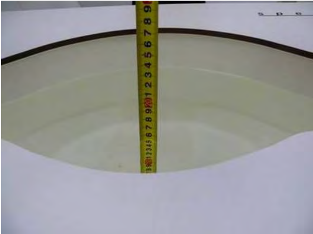
Picture 3: Liquid depth in the Flat Phantom (1750 MHz, 15.3cm depth)
