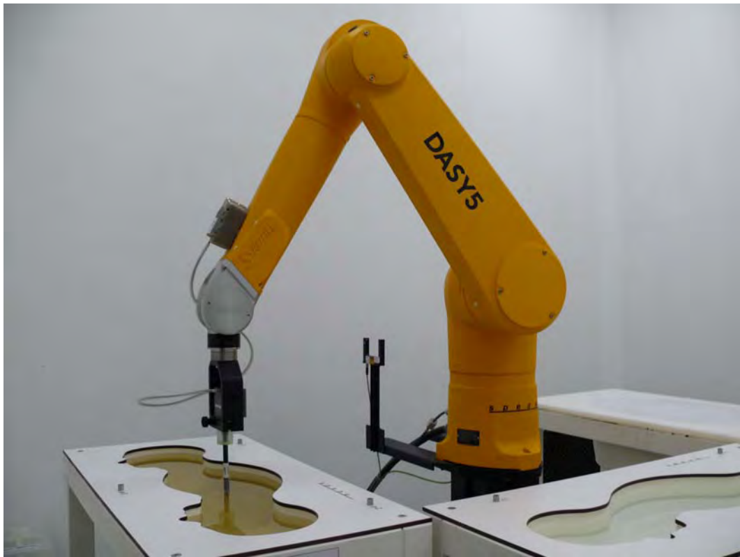
Picture 1: Specific Absorption Rate Test Layout
