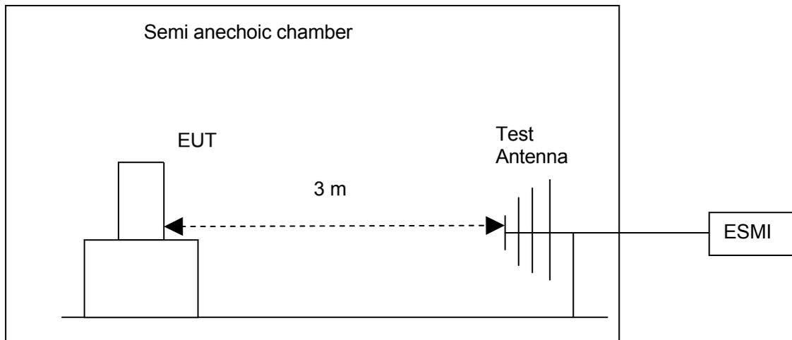
Figure 5. Test set-up
