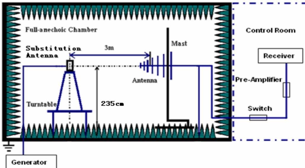
According to part 22.917, the defined measurement bandwidth as following:
