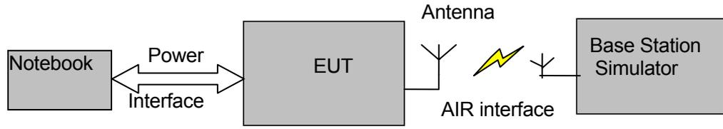
Figure 4. Test Configuration
