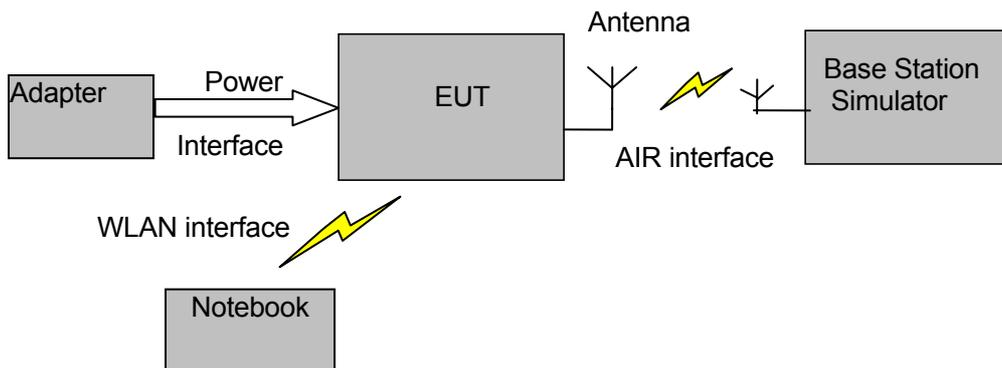
Figure 1.: Test Configuration
