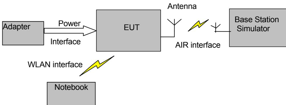
Figure 3. Test Configuration
