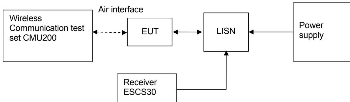
Figure 6. Test Set-up
