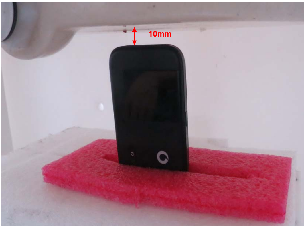
Picture 11: Test Position 3(Original R215)
