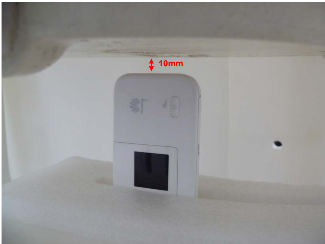
Picture 18: Test Position 4(Variant E5372s-32)
