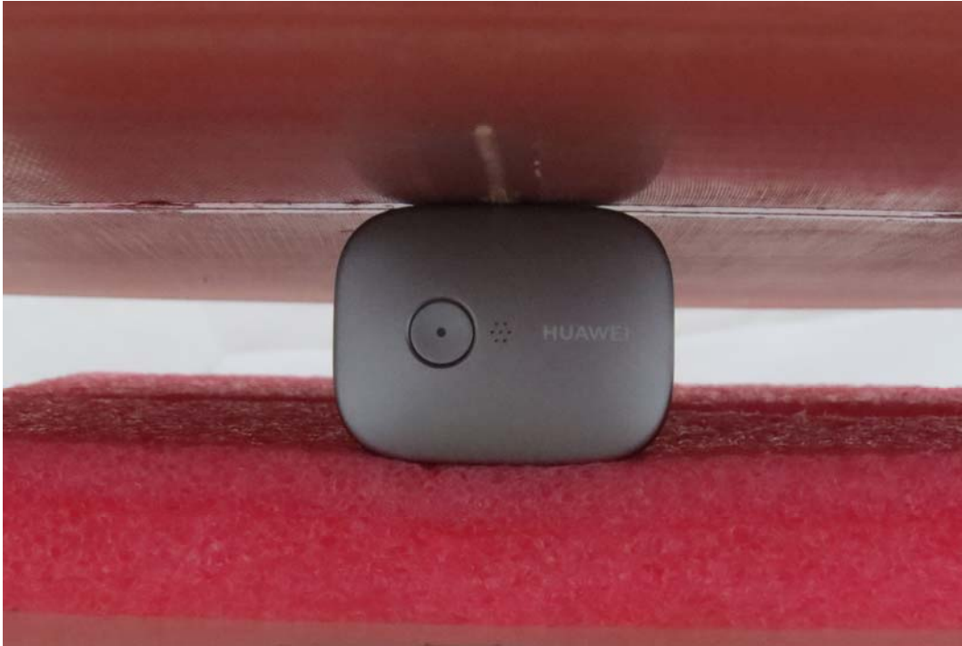
Picture 5: Top Side, the distance from handset to the bottom of the Phantom is 0mm
