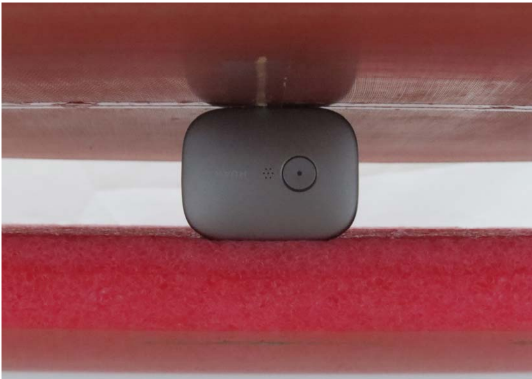
Picture 6: Bottom Side, the distance from handset to the bottom of the Phantom is 0mm
