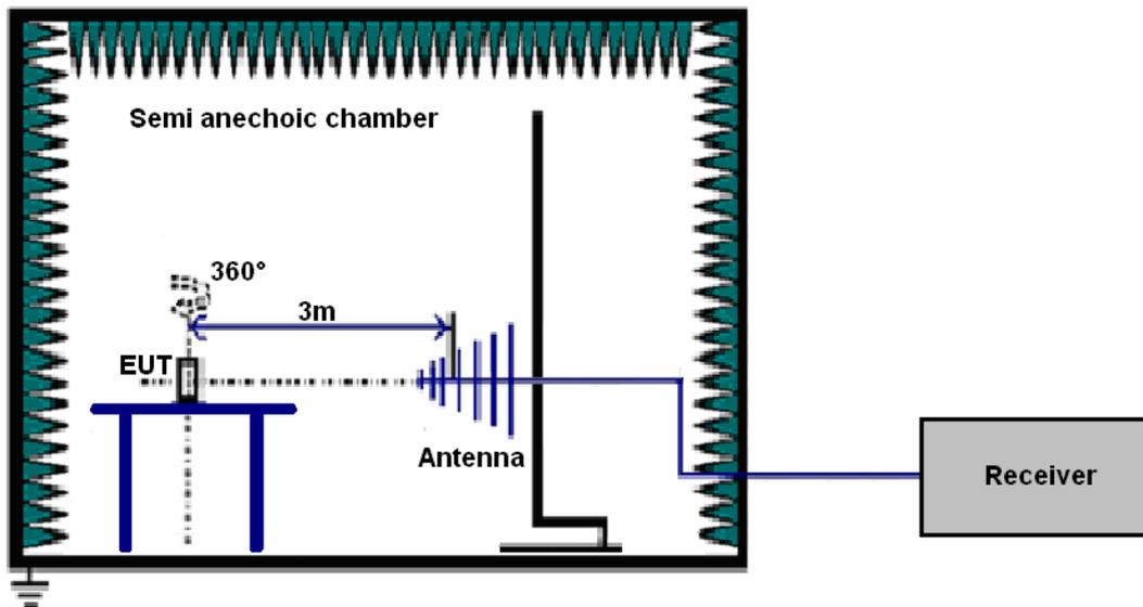
Figure 3. Test set-up
