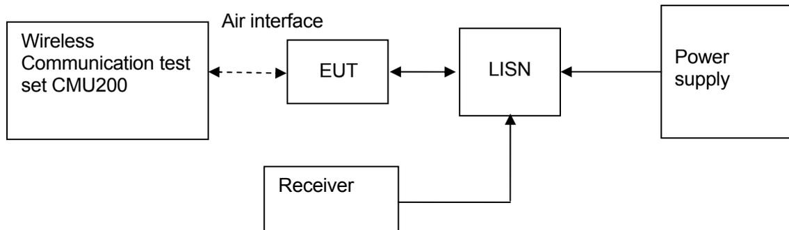
Figure 4. Test Set-up
