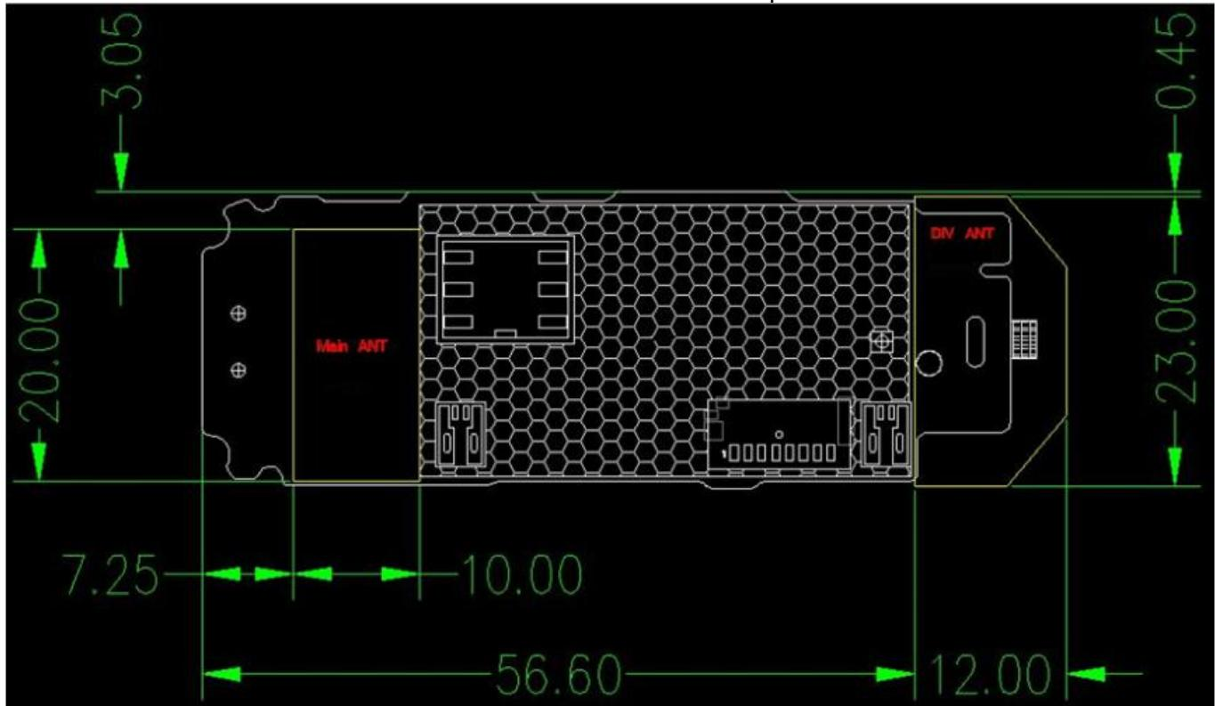
Note : Div antenna is used to improve the acceptance of performance of the main antenna. It does not have the transmitter function.
