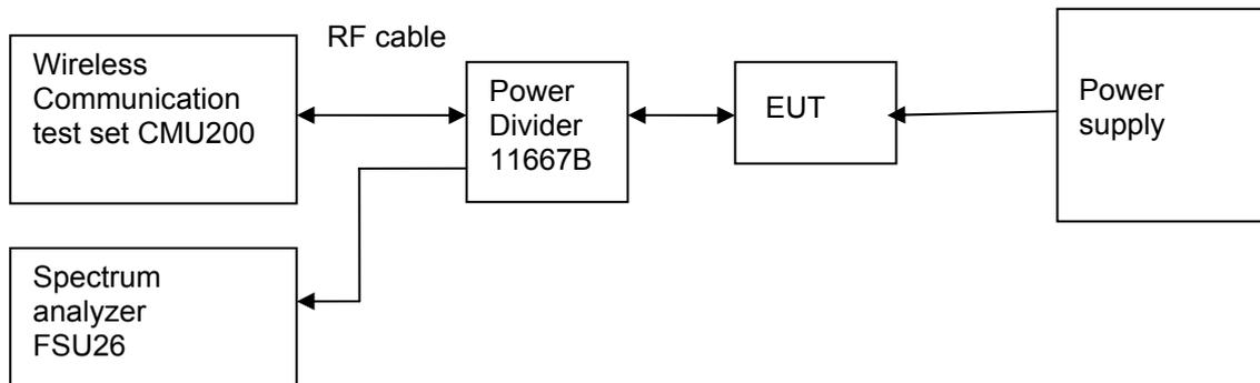
Figure 5. Test Set-up
