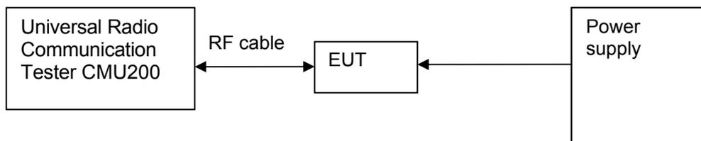
Figure 2. Test Set-up
