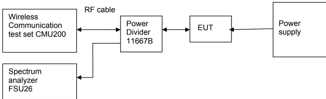
Figure 6. Test Set-up
