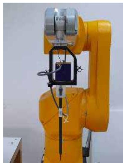
**Figure 3. EX3DV4 E-field probe**
